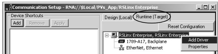
This communication path is used on the PanelView Plus to communicate to the controller in your runtime application in Chapter 8.
