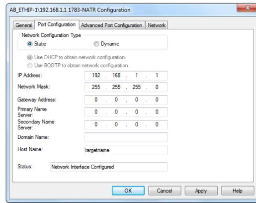
5. For Network Configuration Type, click Static to assign this configuration to the port.
