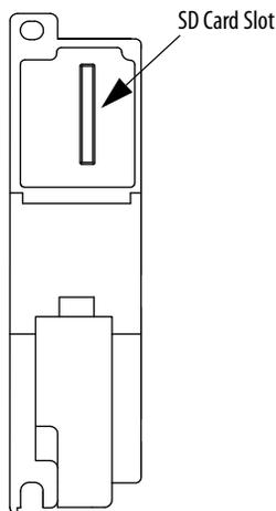
3. Insert the SD card into the SD card slot.
