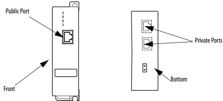
2. Connect one end of an Ethernet cable to the front panel port used as a device port.
