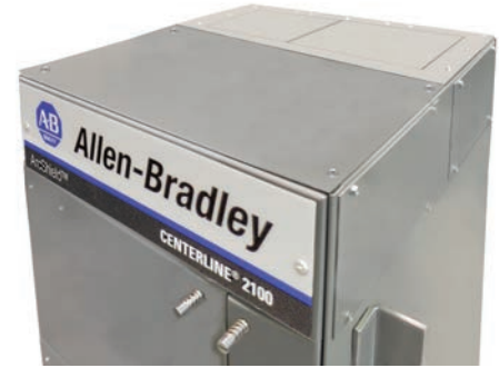
Pressure relief vents allow hazardous gases to escape from the top of the MCC
