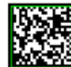
Quiet zone violation
