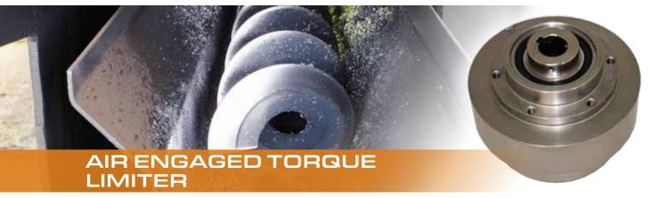
An air engaged torque limiter acts as a clutch to start an auger machine rotation and acts as an overloadsensing device in the event of a jam up in the feed mechanism. The torque limiter is mounted on the driven shaft and coupled to the gear reducer output shaft.
