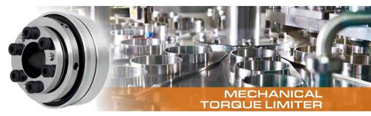
A mechanical torque limiter, installed between the output of a gear reducer and the driven shaft, protects the gear set if an overload happens on the conveyor system. The coupling bores are made specific to the gear box output shaft and main drive shaft. The elastomer transmits torque without backlash or vibration.
