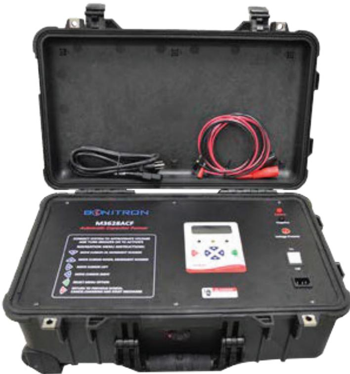
**Measuring aging capacitors helps avoid pre-emptive replacement**
