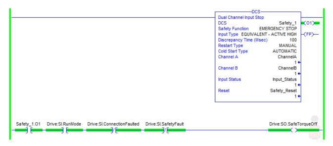
ISO 13849-1 stipulates that instruction reset functions must occur on falling edge signals. To comply with this requirement, a One Shot Falling (OSF) instruction is used on the reset rung. Then, the OSF instruction output bit is used as the reset bit for the **DCS** instruction.
